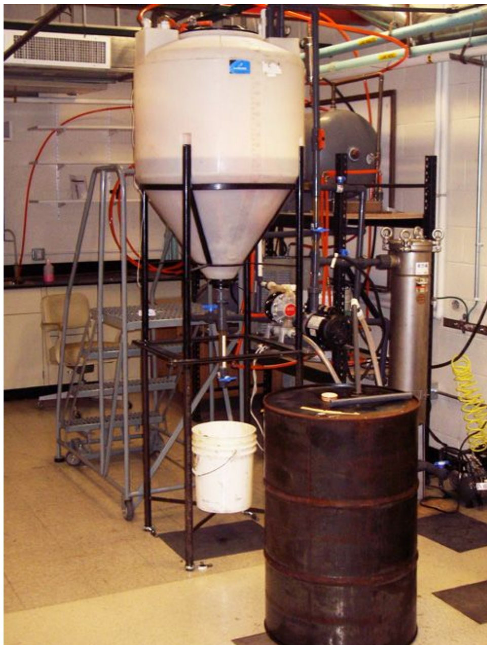
The MIT biodiesel reactor is capable of processing 70-gallon batches of waste vegetable oil into almost the same amount of biodiesel. Here the main processor tank (top center) contains about 20 gallons of biodiesel that was produced from oil collected in a 55-gallon drum (bottom right) at the Student Center.
