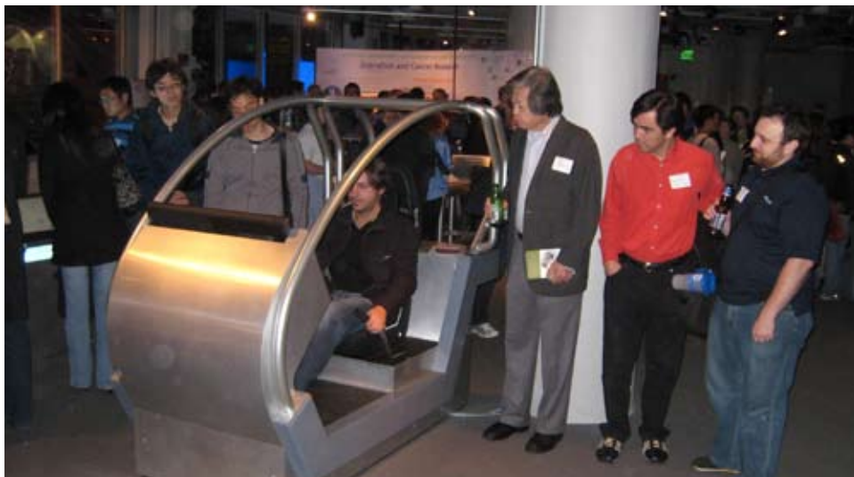
Visitors to Energy Night took turns sitting in a prototype of the MIT Media Lab's City Car, a two-passenger electric vehicle that can be folded, stacked up with others, and recharged at subway stations and other central sites. A passenger arriving by subway or bus simply takes a fully charged vehicle from the front of the stack and then returns it to a stack near his or her destination so that it is available for others to use.
